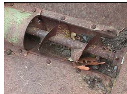
Grain Auger Shear Point Photograph Courtesy of UC Davis
