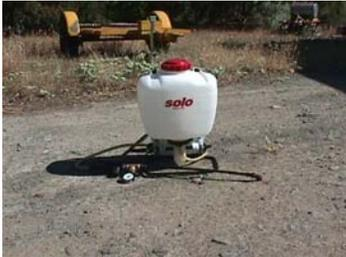
Backpack pesticide sprayers are useful equipment for precisely applying insecticides and herbicides over relatively small areas. Typically, backpack pesticide sprayers hold from four to six gallons of mixed water and chemicals and therefore, fully loaded sprayers weigh from 35 to over 50 pounds. Safe and effective use of a backpack pesticide sprayer is dependent upon accurately applying the proper amount of pesticide.
